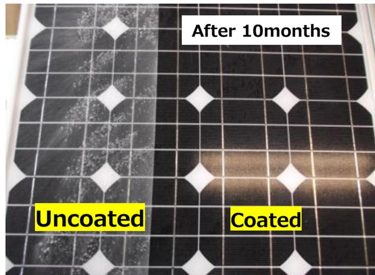
In the desert area where it doesn't rain like the panel in the left picture above, the air is a dry and the sand is charged and easy to adhere. Solar panel glass is required to have a surface that is difficult to adhere.
