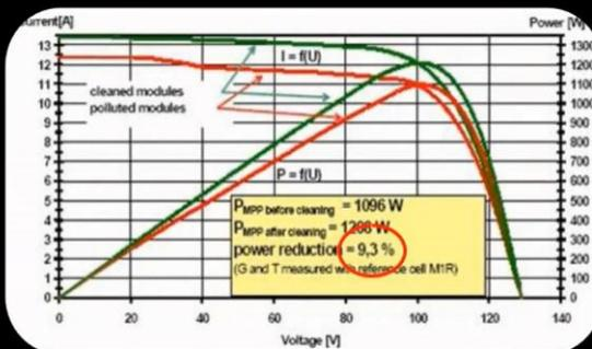
Up to 9.3% reduction in power generation output due to contamination
