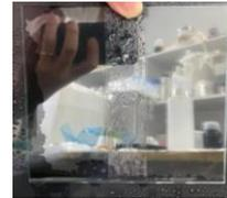
Normally, the glass surface becomes water-repellent (= high water droplet contact angle) when it is splashed with water. SGB can be modified to a hydrophilic state (= low water droplet contact angle) where water spreads on its surface. There are three patterns: when the original hydrophilicity is improved when nanomaterials are added, when there is no change, and when it is decreased.
